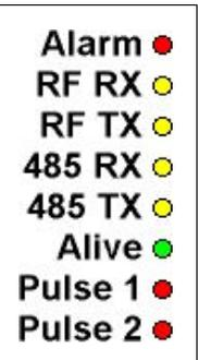
When the ModHopper is operating, the Test Button can be used to report the signal strength received by the ModHopper from another unit. Press and hold the test button. The status LEDs will light up as a bar graph display. Each LED is approximately 10% of scale. For example if PULSE 1 and 2 are on, the received strength is approximately 20% to 29%. For useful signal reporting, it is important to turn off all but one other ModHopper.
