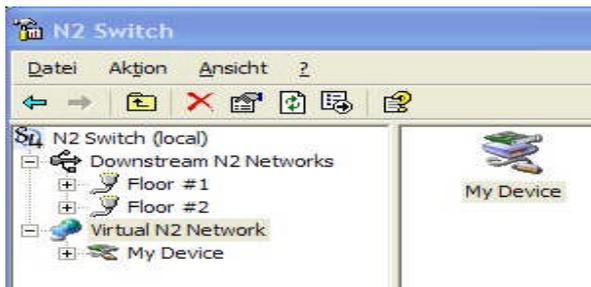
each Downstream N2 Network and publishes the devices, and their associated points, onto the Upstream Virtual N2 Network®. N2 Address translation is applied, wherever necessary, to avoid duplication of N2
