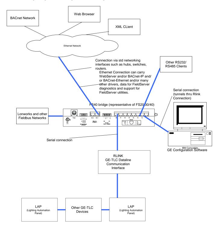
**Appendix C.4.** Cable for Secondary Port (Tunnel) Connection (FS20 and FS40)
