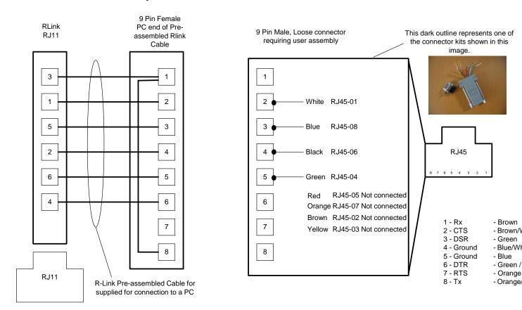
GE-TLC Rlink to FieldServer using pre-assembled GE-TLC Rlink-PC Cable.
