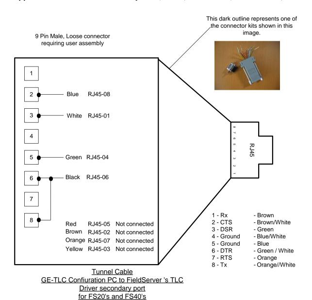
**Appendix C.5.** Cable for Secondary Port (Tunnel) Connection (FS30 Series)
