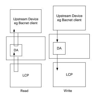
Thus when the upstream protocol writes a '1' to DA\_N22\_Status offset 5 (6<sup>th</sup> location) the driver creates a one shot write to the LCP\_22 and tells it turn relay 6 on. If the upstream device wrote a zero the command to turn relay 6 off would be sent.
